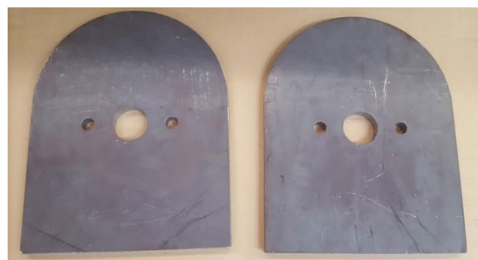
Machined Weight Flats to be used for the counterbalance
